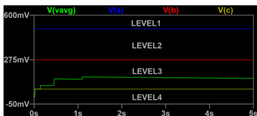
Fig. 15. The output of averaging circuit (green color) exited in level 3 zone
