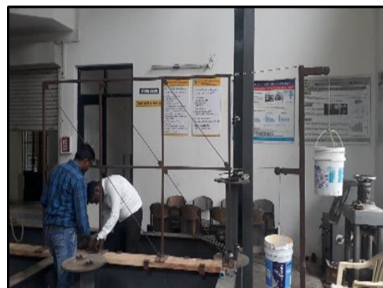
Fig.1.7 Three bays frame with conventional brace.
