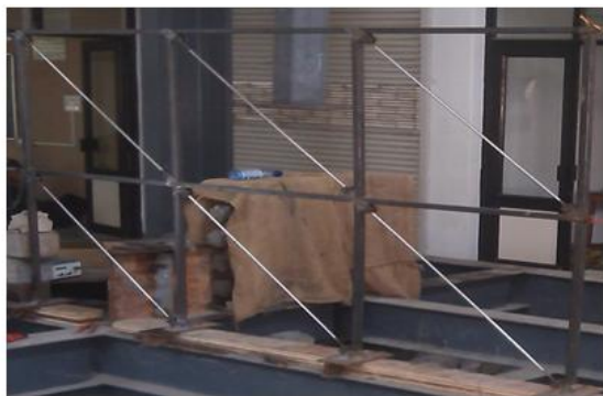
Fig.1.9 Three bays frame with buckling restrained brace
