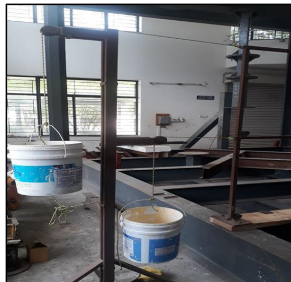
Figure 1.2 Actual Loading Arrangement Following fig.1.3 shows the failed members when loaded with static lateral load
