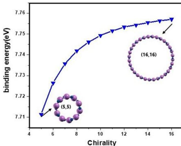
Fig 2. Binding energy of InN nanotube in term of chirality
