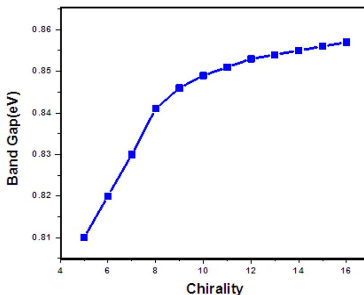
Fig3. Band gaps of InN nanotube in term of chirality
