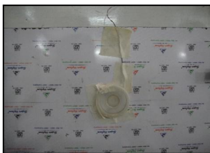
Fig. 4. Load cells (piezoelectric sensors) fixed on mica
