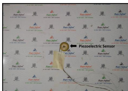
Fig. 4. Load cells (piezoelectric sensors) fixed on mica
