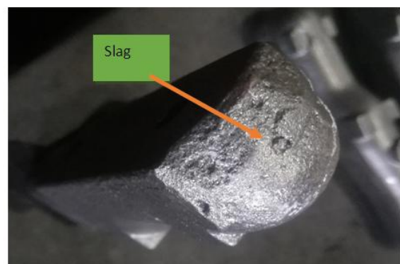
Fig 5: -View of slag inclusion on the product
