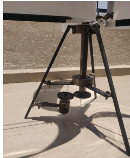
Stand and Generator Gear Arrangement
