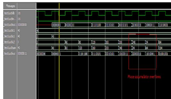
Fig. 11. Simulation result of DDS based on ROM LUT
