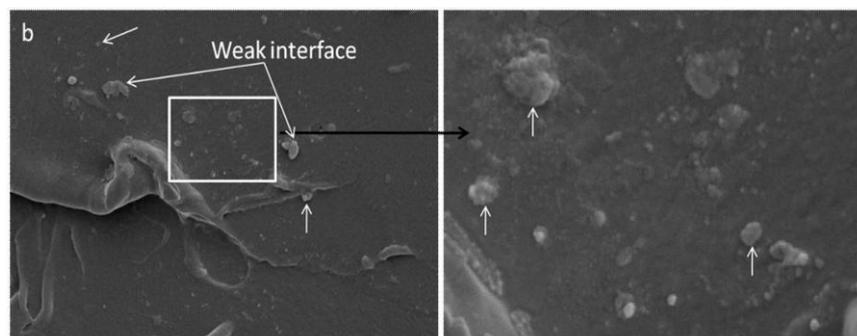
**Figure 4 SEM images of PLA/MgO nanocomposites (nanoparticles are indicated with white arrows; right image is the squared section from left images with magnification).**
