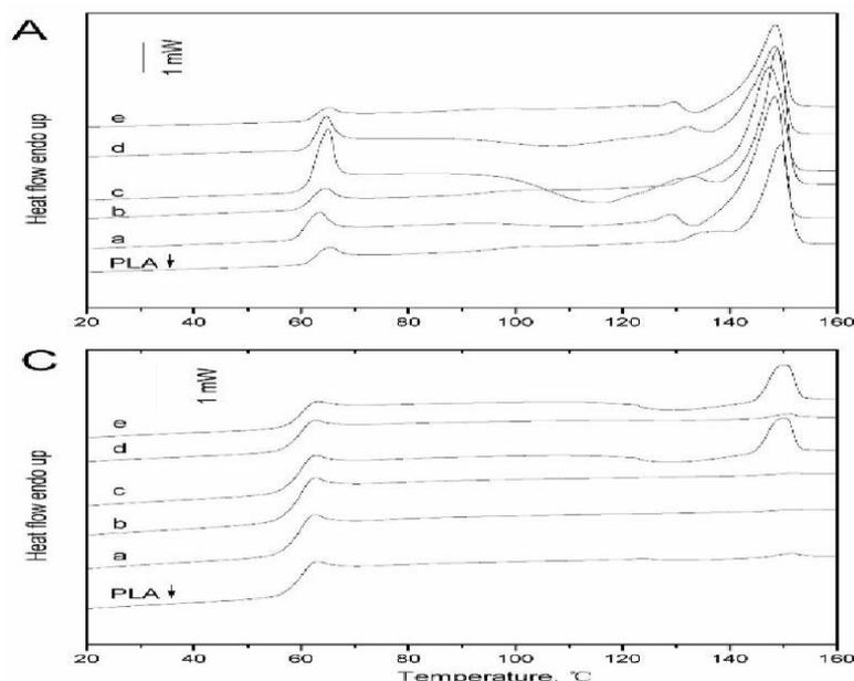
**Figure 5** DSC thermograms of PLA/MgO (A, first scan; C, second scan) nanocomposites with various nanoparticle loading levels (a, 0.0125%; b, 0.025%; c, 0.05%; d, 0.2%; e, 0.8%).
