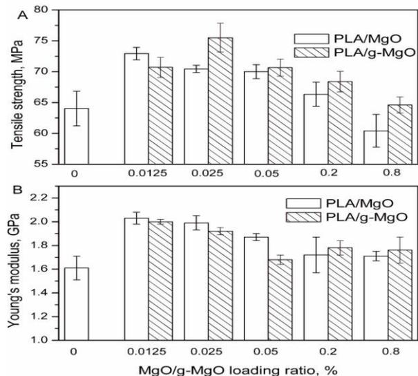
Figure 2 Tensile strength and Young's modulus of PLA/MgO nanocomposites.
