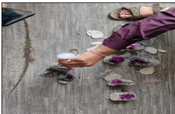
Fig.8 Spraying of Phenolphthalein on core sample
