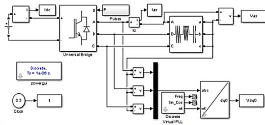
Fig. 7: Simulink model of the inverter supplying RL load
