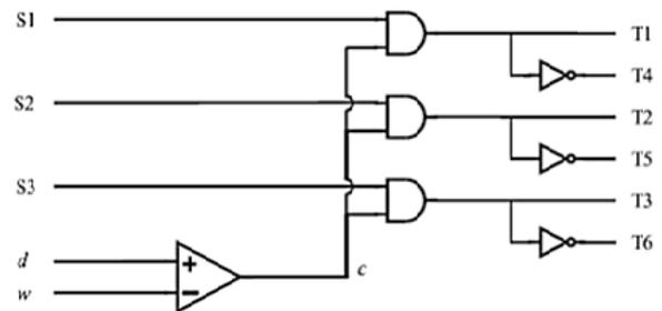
Fig. 2: Switching pulse generating circuit for six-step modulation
