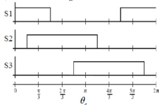
Fig. 3: Signals S1 – S3 as functions of  $\theta_c$
