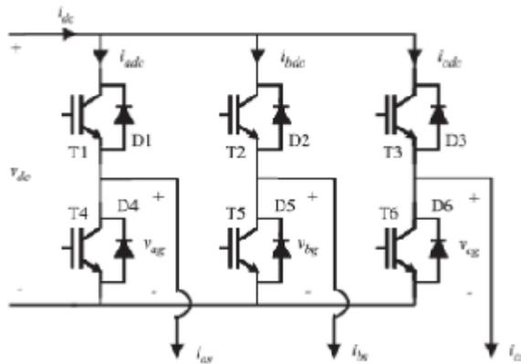
Fig. 1: Three-phase bridge converter connection
