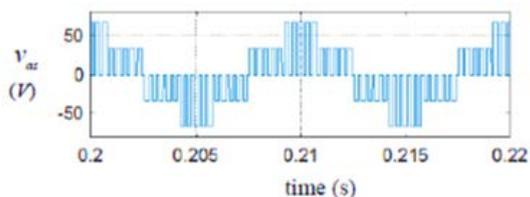
Fig. 8: Load voltage versus time for six-step modulation
