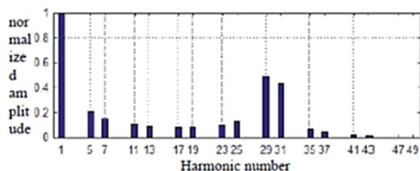
Fig. 9: Frequency spectrum for six-step modulation
