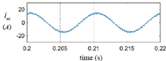
Fig. 16: Load current versus time for sine-triangle modulation
