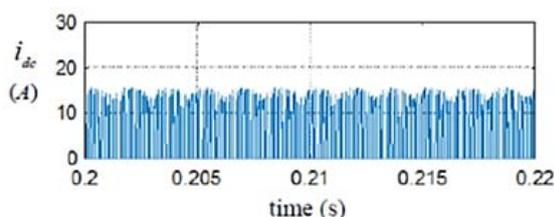
Fig. 17: DC current versus time for sine-triangle modulation
