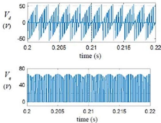
Fig. 15:  $V_d$  and  $V_q$  versus time for sine-triangle modulation
