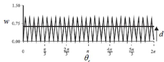
Fig. 4: The duty cycle and signal  $w$  as functions of  $\theta_c$
