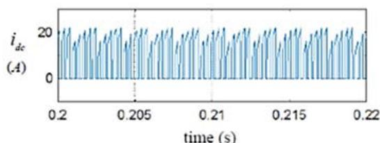
Fig. 12: DC current versus time for six-step modulation
