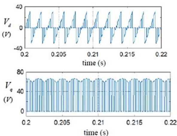
Fig. 10:  $V_d$  and  $V_q$  versus time for six-step modulation
