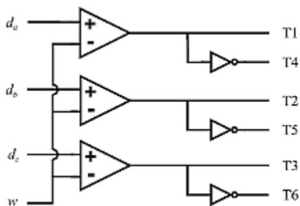
Fig. 5: Switching pulse circuit for sine-triangle modulation
