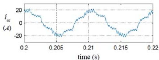
Fig. 11: Load current versus time for six-step modulation
