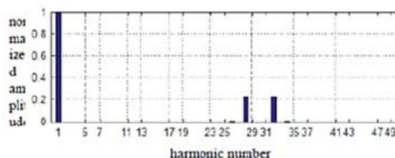
Fig. 14: Frequency spectrum for sine-triangle modulation
