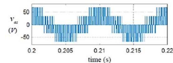
Fig. 13: Load voltage versus time for sine-triangle modulation
