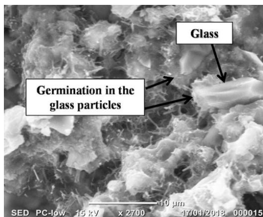
Fig. 3. SEM image of C-S-H germinating from glass microparticles in a mortar containing 30% replacement of cement by glass after 90 days of curing [37].
