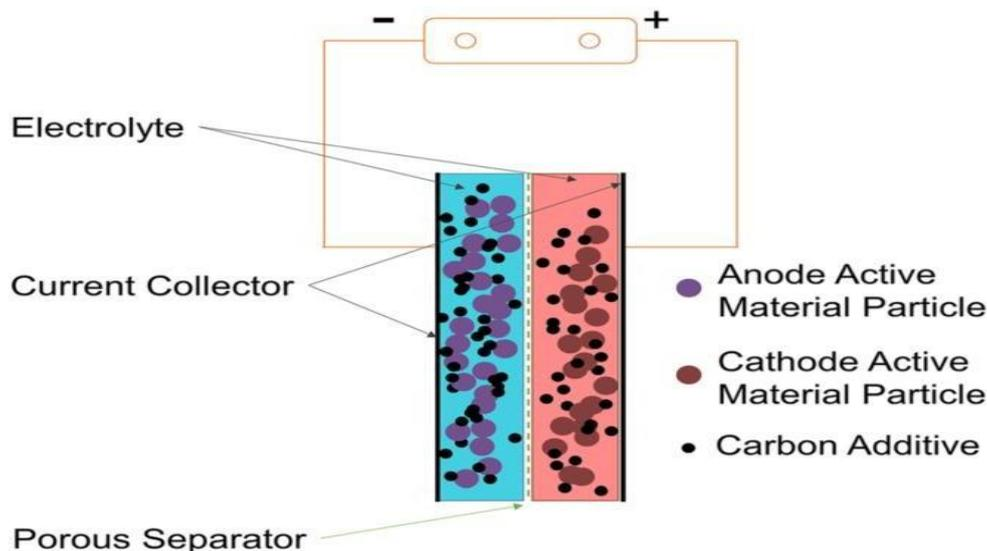
Fig.1: Lithium-ion battery
