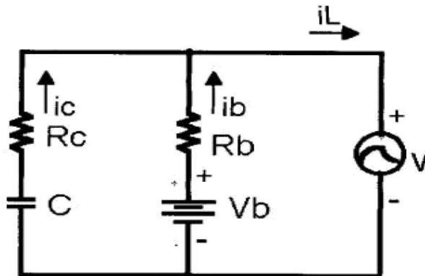
Fig.4 System Circuit
