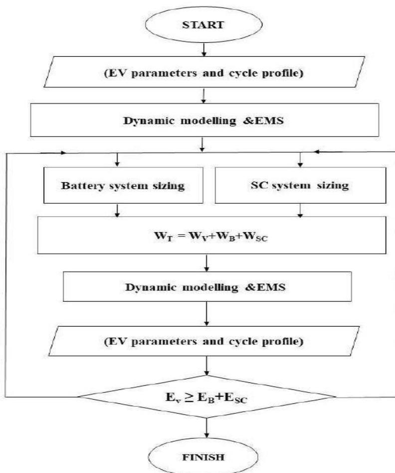
Fig.3- System Sizing Algorithm
