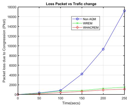
Figure 6. Cumulative packet loss as the source of information increases
