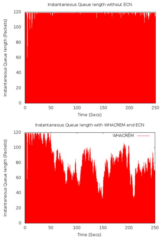
Figure 9. Instant queue when router with and without ECN
