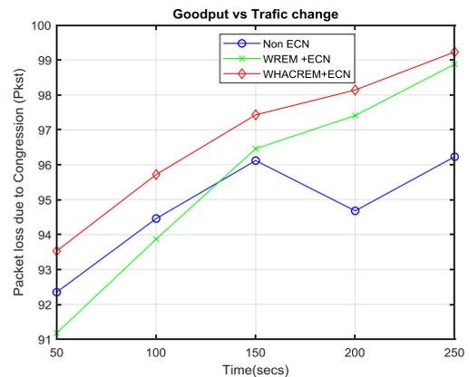
Figure 8 Goodput when a router with and without using ECN
