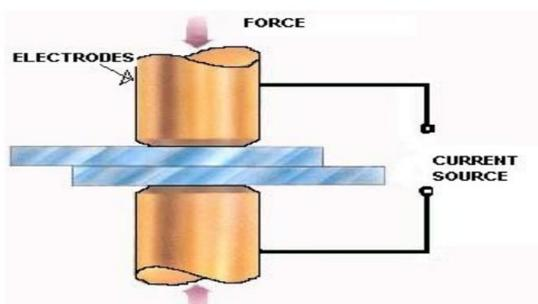
In spot welding, two sharp copper alloy electrodes are used to cluster the welding current to a petite 'spot' as well as fasten the work pieces simultaneously. Inflicting a sizeable current via the two metal pieces eventually melt them a bit for welding. The best part of this procedure is that it occurs very quickly, in just 10 milliseconds and that too to a specific small spot to which the heat generated is not too much to result in warping.
