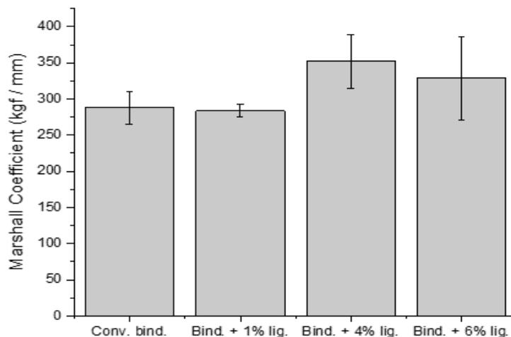
**Figure 4:** Marshall coefficient for the sample of conventional and modified lignin binder.
