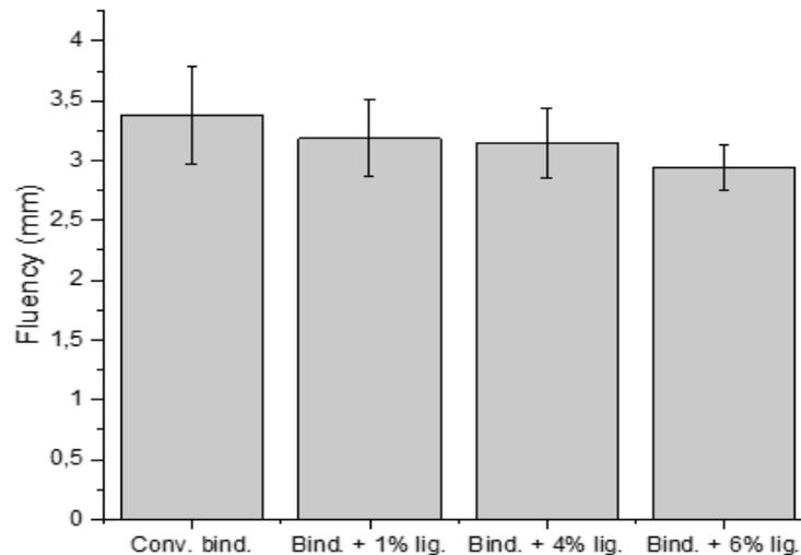
Figure 3: Marshall fluency of conventional binder and lignin-modified binder
