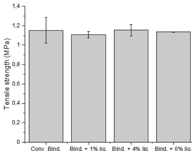
**Figure 5:** tensile strength by diametrical compression of conventional binder and lignin- modified binder.
