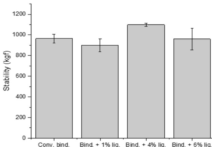
**Figure 2:** Marshall stability of conventional ligand and lignin-modified ligand.
