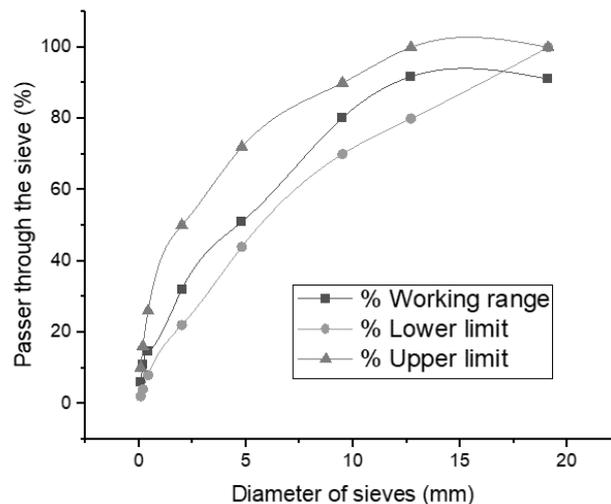
Figure 1: granulometric analysis of this work based on the DNIT-ES 031/2006 Brazilian Standard
