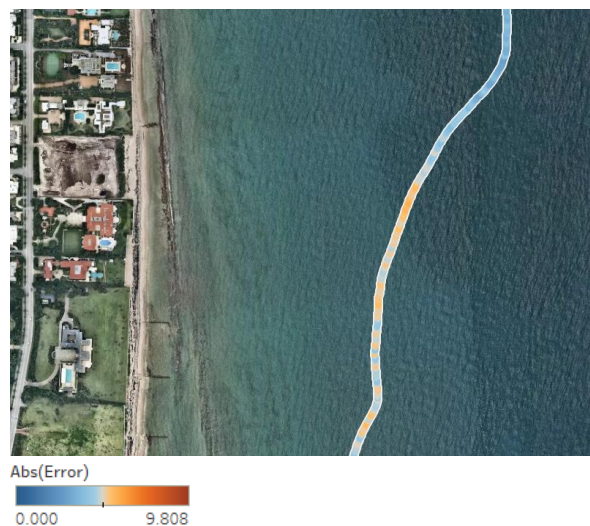
Figure 8. Comparison of measurements and predictions for Wi-Fi Channel 6 (Calibration data)
