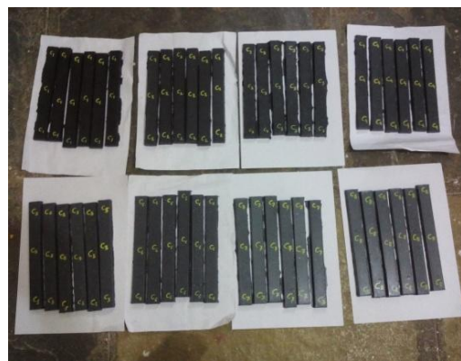
Fig 2.2 Composite Specimen for Mechanical Testing filled with Graphite & TiO_2
