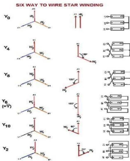
Figure 2 – Various ways to wire Star winding.
