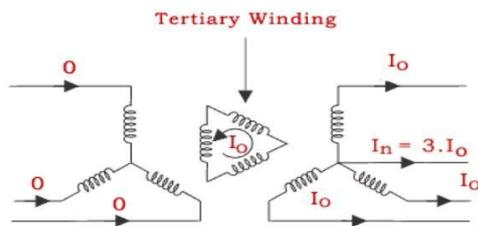
Diagram of Three Winding Transformer
