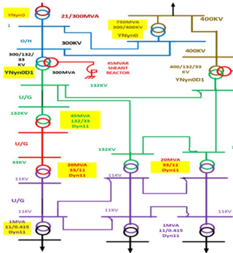
Figure 3 – Transformer Distribution through Electrical Network.
