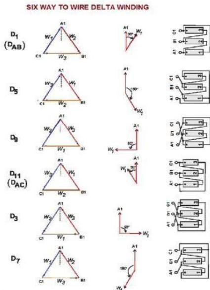
Figure 1 – Various ways to wire Delta winding.
