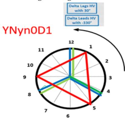
Figure 5 – Clock notation for **YNyn0D1** Transformer
