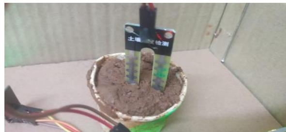
Figure 6 Soil Moisture Sensor
