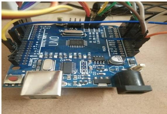
Figure 2. Arduino Uno Board
