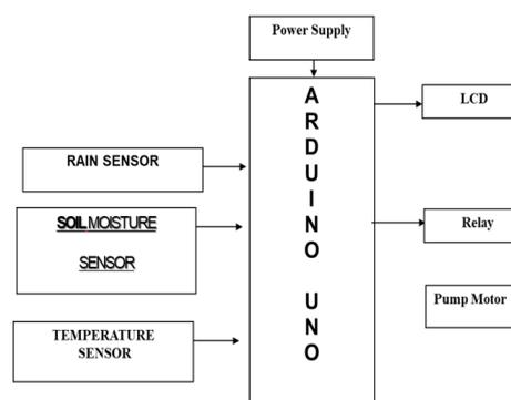
Figure 11. Interfacing of Devices
