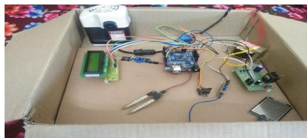
Figure 17 Interfacing of all Sensors with Arduino Board
