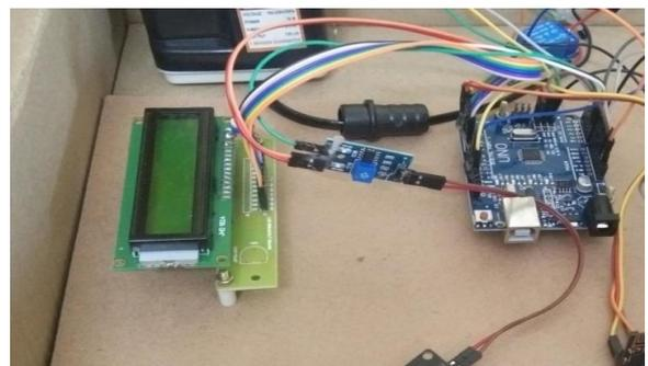
Figure 16 Interfacing of Arduino with LCD
