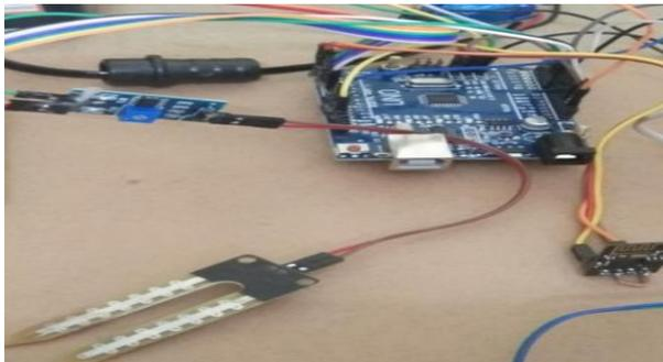
Figure 13 Interfacing of Soil Moisture Sensor
