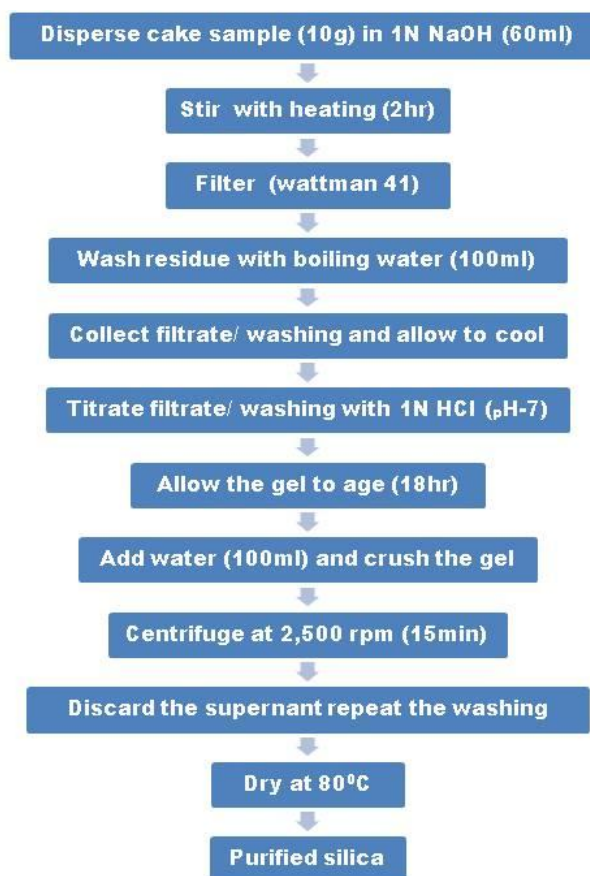
Figure 1 Flow chart of procedure used for Silica extraction
