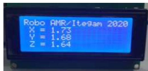
Figure 14 - LCD showing the information obtained from the Beacon. Source: Authors, (2021).
