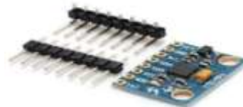
Figure 1 - Accelerometer and 3-axis Gyroscope MPU - 6050. Source: [53].
