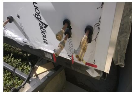
FIG. 9 View of the possibility of connecting a mobile laboratory to an external heat source [Photo source: authors]
