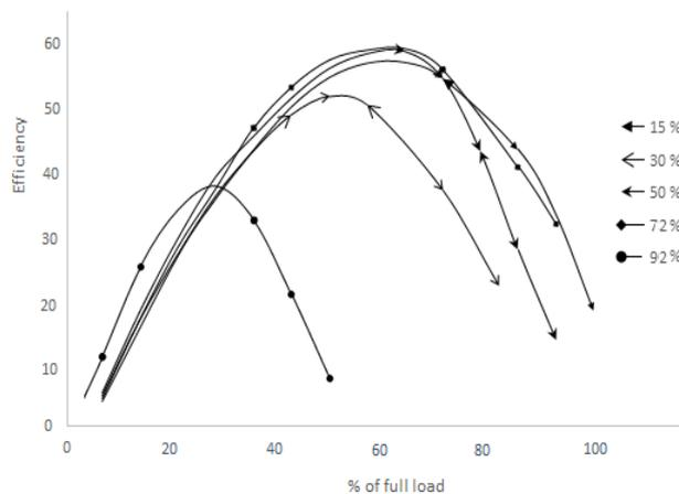
**FIGURE 5.** Variation of efficiency ( $\eta$ ) with % of full load at various wicket gate opening
