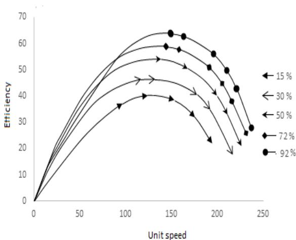
**FIGURE 4.** Variation of efficiency ( $\eta$ ) with unit speed ( $N_u$ ) at various wicket gate opening
