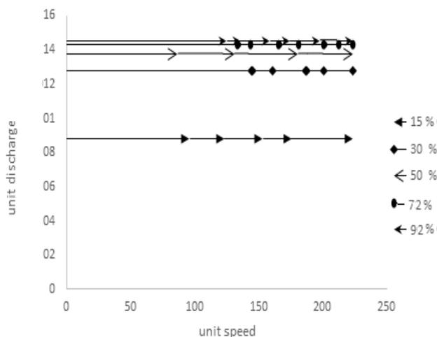
**FIGURE 2.** Variation of unit discharge ( $Q_u$ ) with unit speed ( $N_u$ ) at various wicket gate opening
