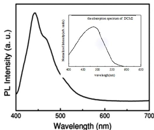
Figure 3: The photo-luminescence spectrum of FIrpic and the absorption spectrum of DCM2 in the inset.
