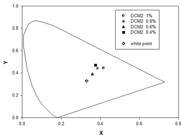
Figure 4: The CIE coordinates of OLED with various DCM2 doping concentration.
