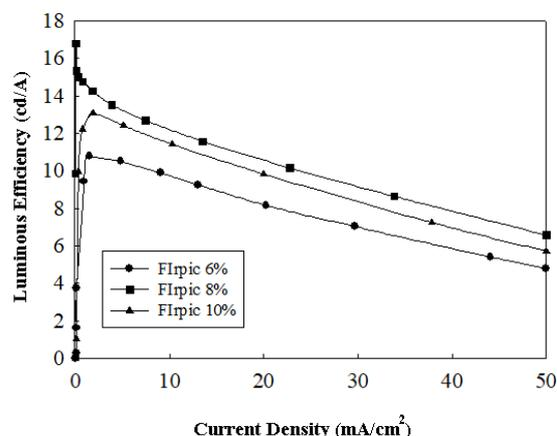
Figure 1: Luminous efficiency - current density characteristics of OLEDs against the doping concentration of FIrpic in CBP.
