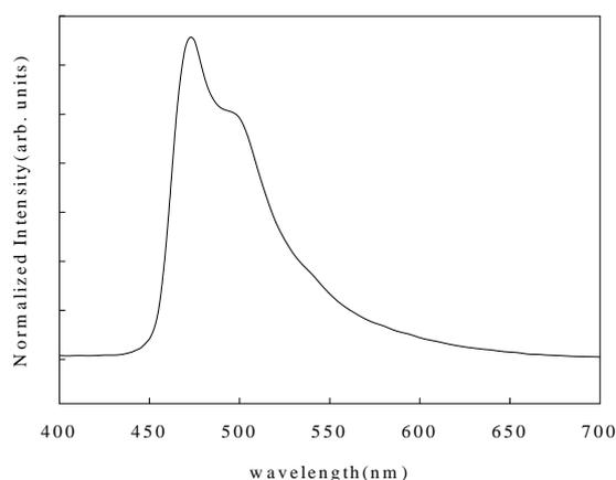
Figure 2: The electroluminescence spectrum of PHOLED with FIrpic as the dopant.
