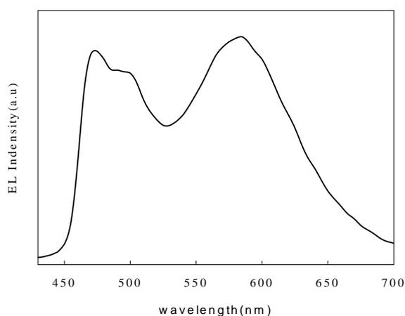
Figure 5: The normalized EL spectrum of white OLED device.
