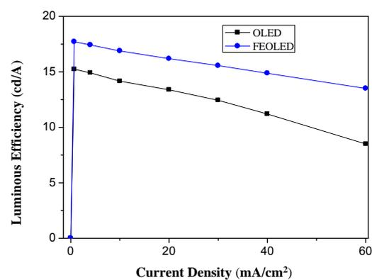
Figure 7: Luminous efficiency – current density of both OLED and FE-OLED devices.
