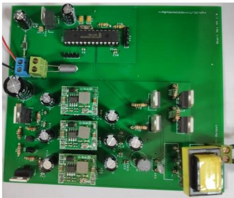
Fig. 12. The fabricated circuit of the proposed High Voltage Supply
