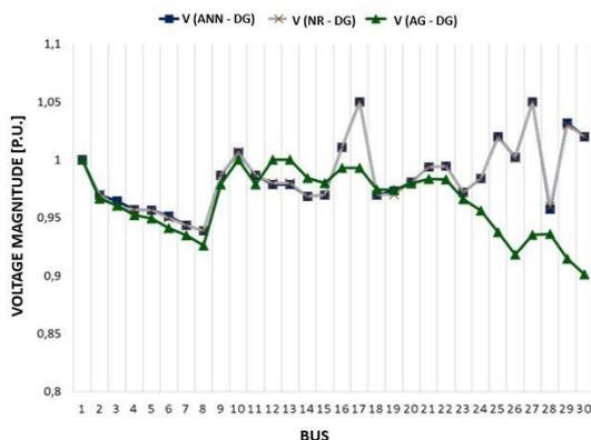
Fig. 6 Comparison between Voltage Magnitudes for the methods applied to the IEEE-30 bus system.
