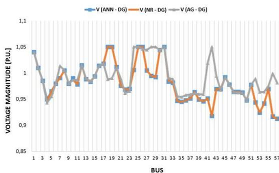
Fig. 11 Voltage magnitudes for the IEEE-57 system with insertion of DGs.
