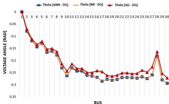
Fig. 7 Comparison between voltage angles for the methods applied to the IEEE-30 bus system.
