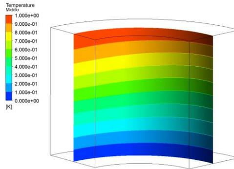
**Figure 5:** isothermal lines of flow inside the cavity
