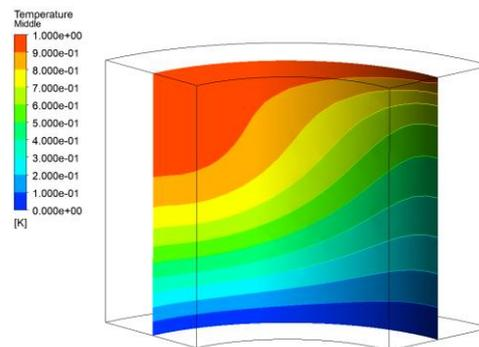
**Figure 7:** isothermal lines of flow inside the cavity
