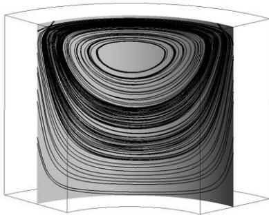
**Figure 3:** Streamlines of flow inside the cavity
