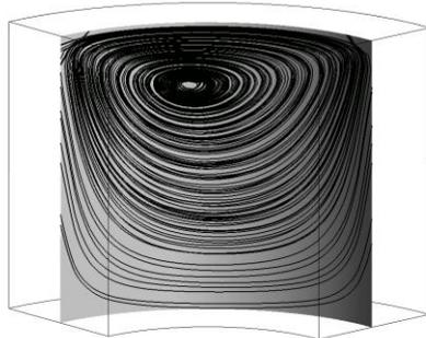
**Figure 4:** Streamlines of flow inside the cavity
