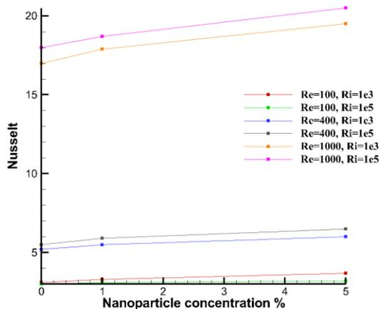
**Figure 8:** Effect of nanoparticle mass concentration, Re and Ri on the Nusselt number of the top wall
