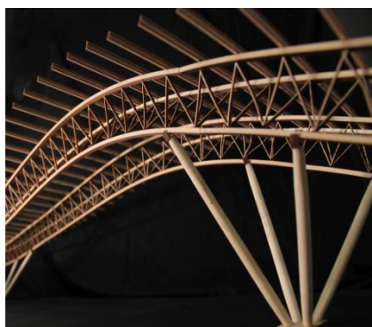
Transformation of load from roof structure to columns
