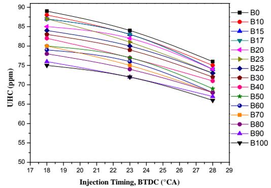
Figure 6. UHC results at different injection timings
