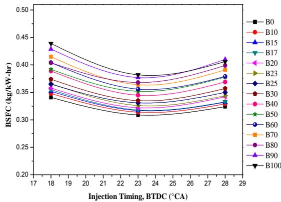
Figure 3. BSFC results at different injection timings
