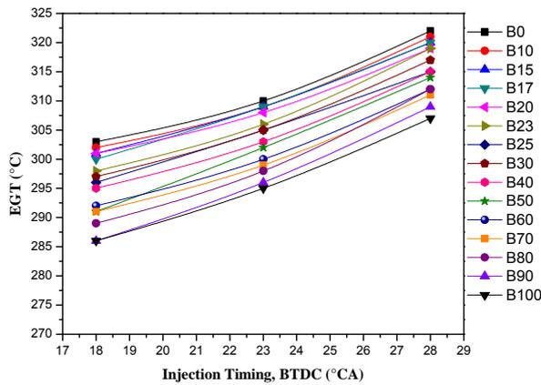
Figure 4. EGT results at different injection timings
