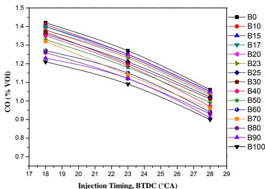
Figure 5. CO results at different injection timings
