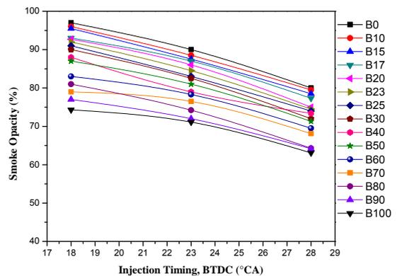
Figure 8. Smoke Opacity results at different injection timings
