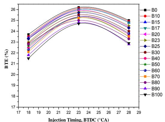
Figure 2. BTE results at different injection timings
