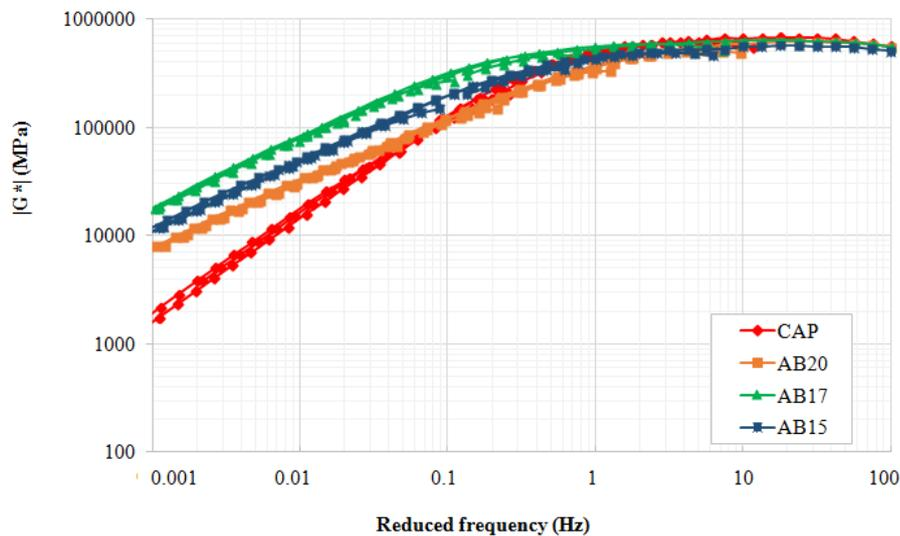
Fig. 8. Master curves of the asphalts.
