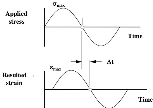
Fig.1. Applied stress and resulted strain for viscoelastic materials (Based on SHRP [10]).
