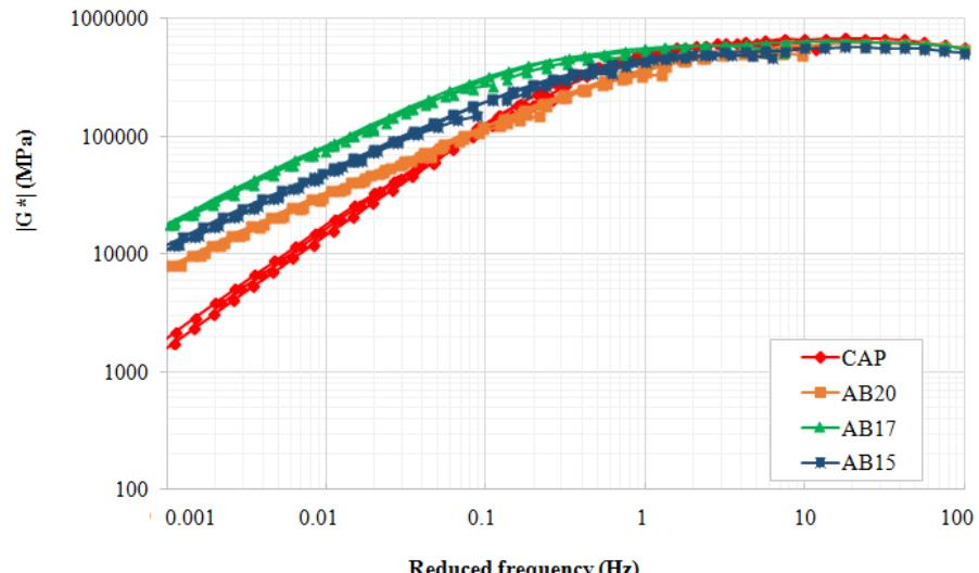
**Fig. 8.** Master curves of the asphalts.
