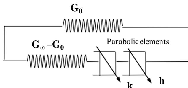
Fig. 3. Huet-Sayegh model (Based on Xu and Solaimanian [16]).
