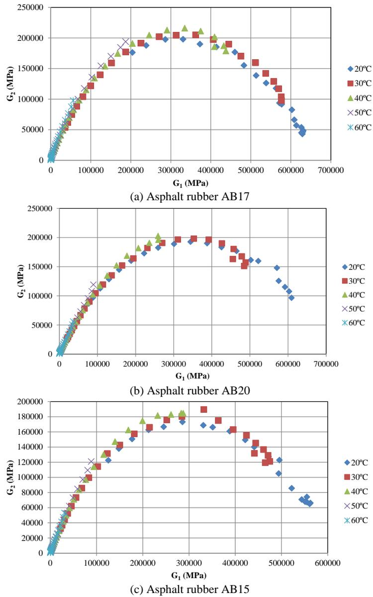
**Fig. 6.** Curves in the Cole-Cole plane for asphalt rubber.
