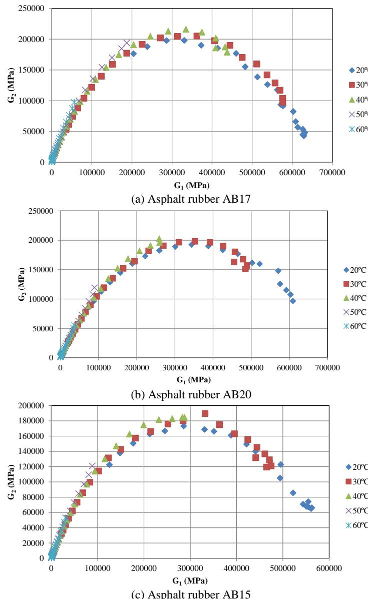
**Fig. 6.** Curves in the Cole-Cole plane for asphalt rubber.
