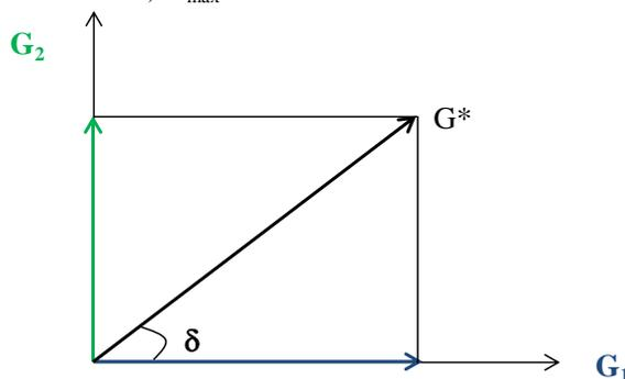
Fig. 2. Complex shear modulus components.
