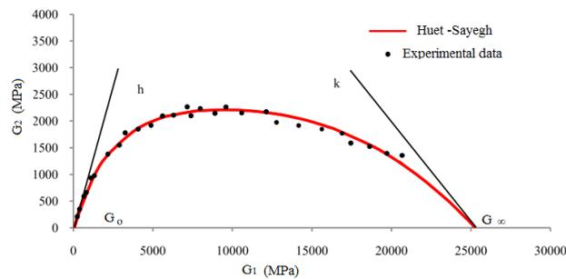
Fig. 4. Huet-Sayegh model adjusted in Cole-Cole plan (Based on Quintero [21]).
