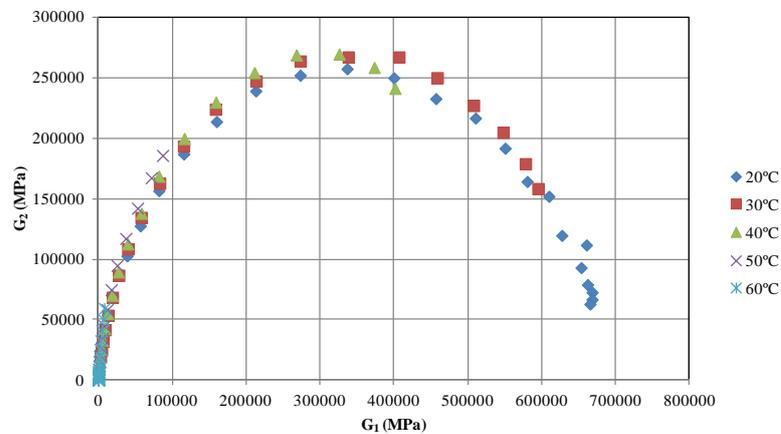
**Fig. 7.** Curve in the Cole-Cole plane for conventional asphalt (CAP).
