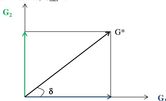
**Fig. 2.** Complex shear modulus components.
