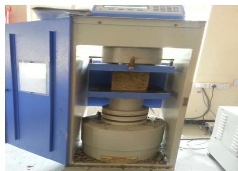
Figure 3: Cube compressive testing on hardened concrete
