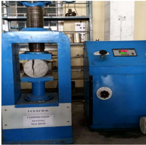
Fig 6.2 Split tensile test specimen of conventional concrete prism
