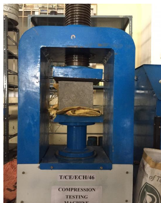
Fig 6.1 Compressive test specimen of conventional concrete cube
