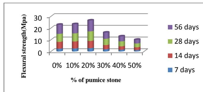
**Graph showing flexural strength of pumice & fibers**
