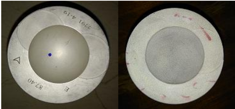
Figure 3. Piston before coating and after coating
