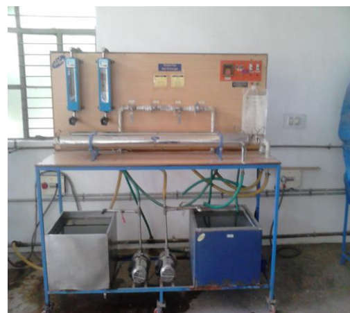
fig 1 Experimental setup of Double Pipe Heat Exchanger
