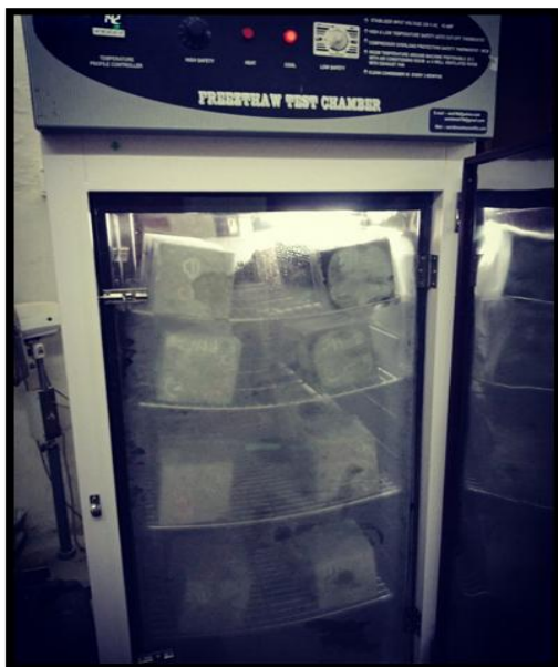
Figure 3. 18: Freeze Thaw Chamber and Freeze Thaw cycle
