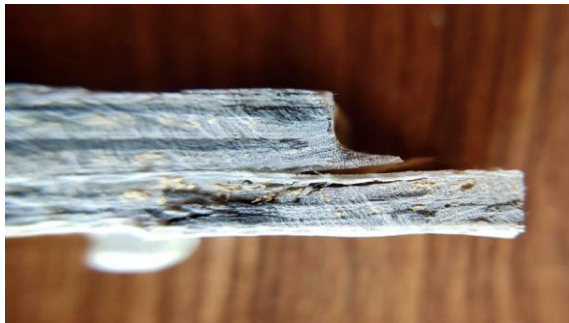
Figure 38: Specimen after Impact test
