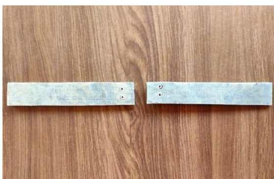
Figure 33: Specimen after tensile test
