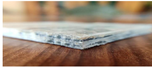
Figure 40: Test specimen for Hardness test
