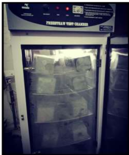
Figure 3. 18: Freeze Thaw Chamber and Freeze Thaw cycle
