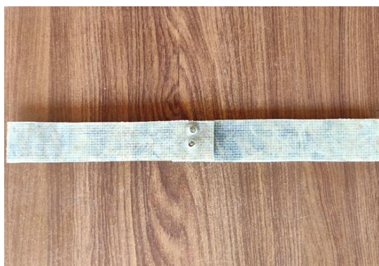
Figure 32: Specimen for Tensile test
