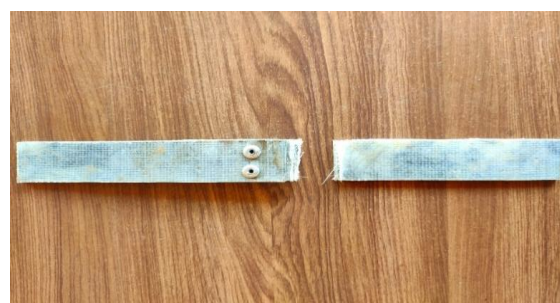
Figure 35: Specimen after bending test
