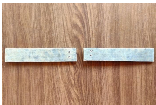
Figure 33: Specimen after tensile test
