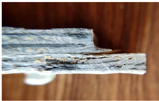
Figure 38: Specimen after Impact test
