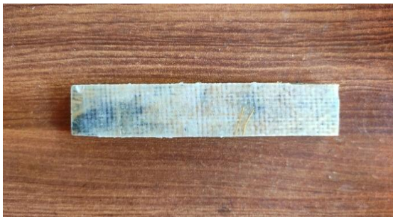
Figure 39: Test specimen for Thermal conductivity test
