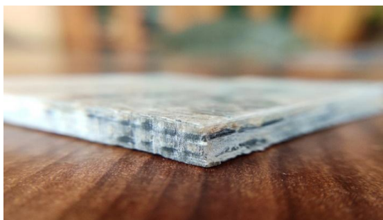
Figure 40: Test specimen for Hardness test
