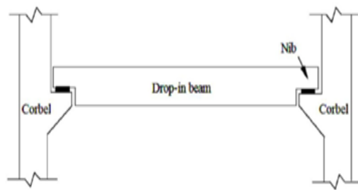
b. Drop-in-Beam supported by Corbels
