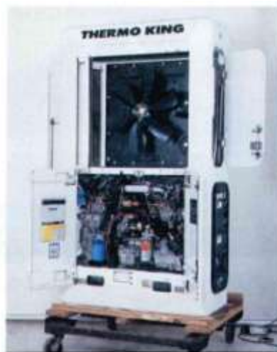
Figure 27-14 Access for service for a nose-mount unit. Courtesy Thermo King Corp.
