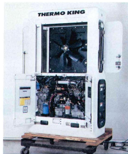
Figure 27-14 Access for service for a nose-mount unit. Courtesy Thermo King Corp.
