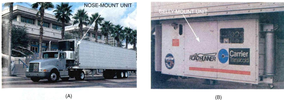
Figure 27-9 (A) Nose-mount and (B) belly-mount refrigerated truck. Reproduced courtesy of Carrier Corporation
