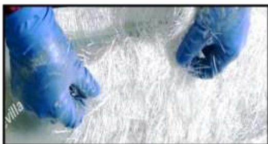
Figure 7. Putting different fiber diameters in the mold with different position angles
