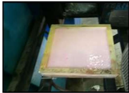
Figure 4. Silicon rubber mold during curing
