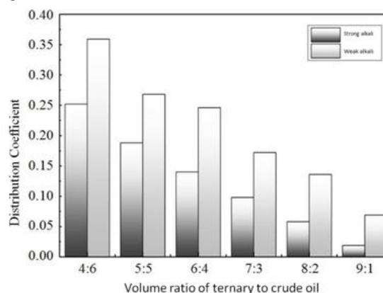
**Fig.3 The effect of strong base and weak base on the distribution coefficient of surfactant in oil phase**
