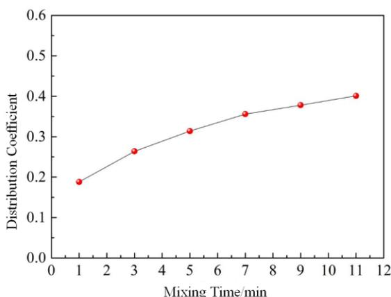
**Fig.1 The effect of stirring time on the distribution coefficient of surfactant in oil phase**
