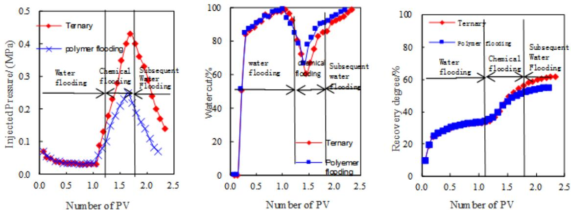
**Fig.5 The relationship between injection-pressure, water cut, recovery percent and pore volume**
