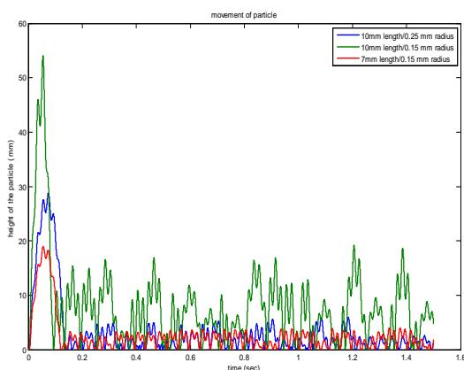
Figure. 2 Radial Movement Cu/ 100KV superimposed of 1050 KV / 55mm - 150mm Enclosure
