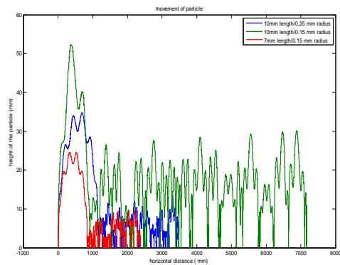
Figure.11 Axial Movement for Cu/ 132 KV superimposed of 1050 KV / 55mm - 150mm Enclosure
