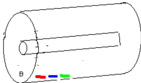
**Figure. 1** Typical single phase gas insulated bus
