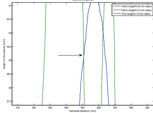
Figure.9 Particle collision for Cu/ 200 KV superimposed of 1050 KV / 55mm - 150mm Enclosure
