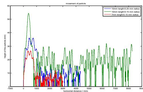
Figure.12Axial Movement for Cu/ 145 KV superimposed of 1050 KV / 55mm - 150mm Enclosure
