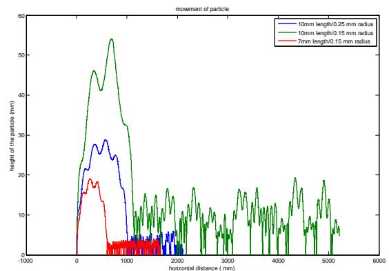
Figure.10 Axial Movement for Cu/ 100 KV superimposed of 1050 KV / 55mm - 150mm Enclosure
