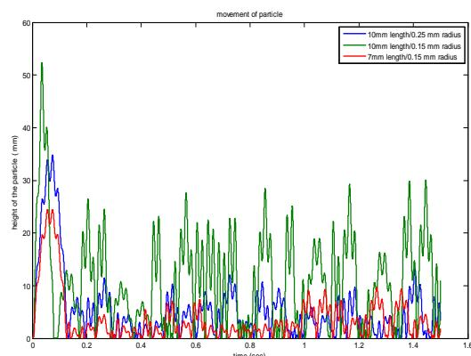
Figure. 3 Radial Movement for Cu/ 132KV superimposed of 1050 KV / 55mm - 150mm Enclosure
