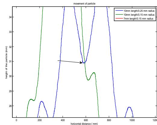
Figure.8 Particle collision for Cu/ 145 KV superimposed of 1050 KV / 55mm - 150mm Enclosure
