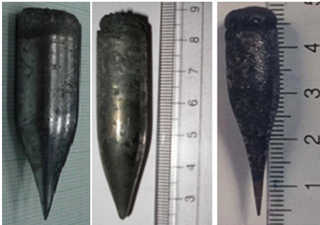
Figure-2 The as grown ingots of \text{In}_{(1-x)}\text{Ga}_x\text{Sb} , a) IGS-1 ( x=0.1 ), b) IGS-2 ( x=0.15 ), c) IGS-3 ( x=0.25 ). The surfaces are without growth morphology, at the beginning concave and the end growth convex..
