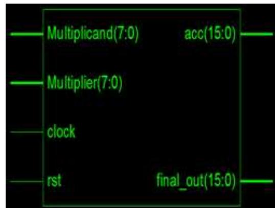
Fig 4: Top Module-Symbol of Multiplier
