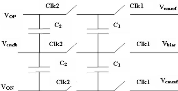
Fig.4. switched capacitance common mode feedback circuit
