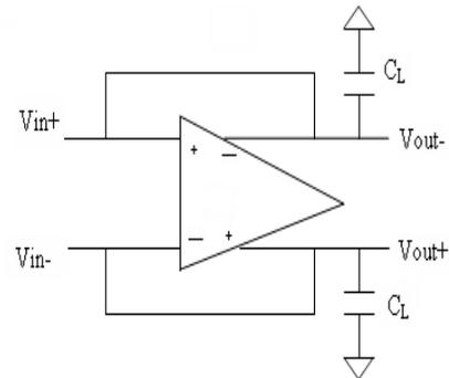
Fig.8. configuration for simulating the step response
