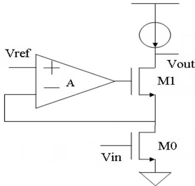
Fig.1. design of the gain-boosted amplifier
