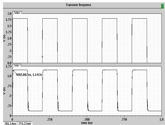
Fig.9. step response of proposed folded-cascode opamp.
