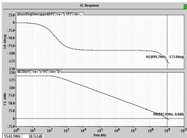
Fig.7. gain and phase response of folded cascode opamp.
