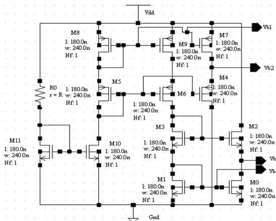
Fig.6. wide swing cascode current mirror circuit
