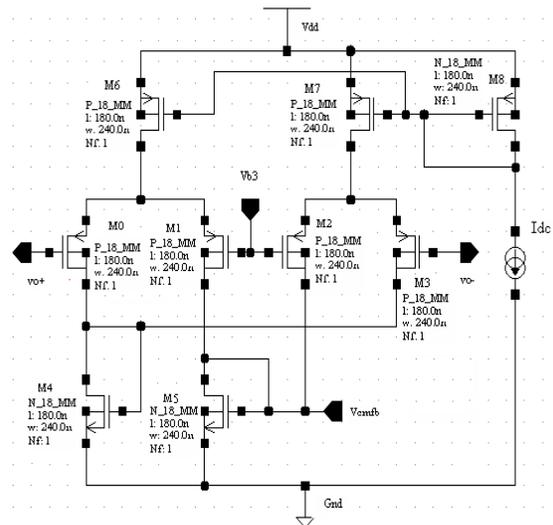
Fig.5. CMFB circuit for gain boosting amplifier AP.
