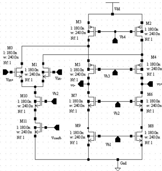
Fig.3. fully differential gain-boosted amplifier (AP).
