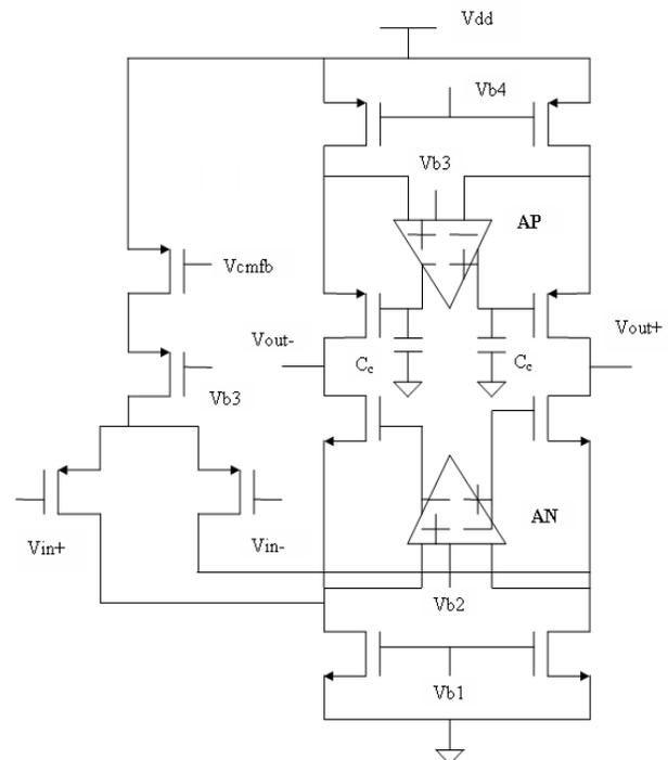
Fig.2. fully differential folded cascoded op-amp with fully differential gain-boosted amplifiers.
