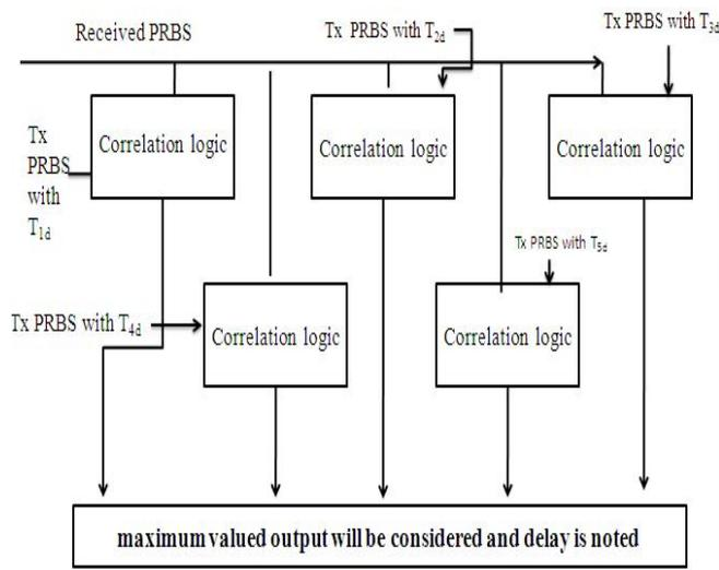
Figure 3: Block Diagram of Digital Correlator with five correlation logics.
