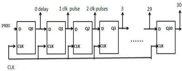
Figure 2: Serial in Parallel out Shifter
