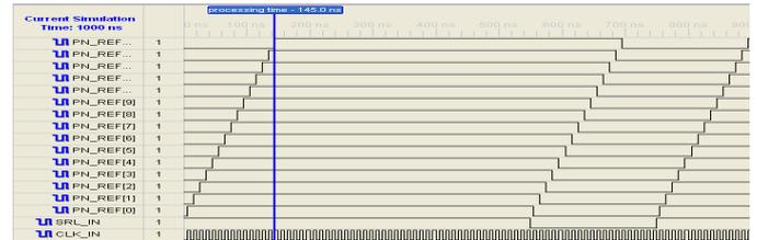
Figure 5: Delayed versions of transmitted PRBS
