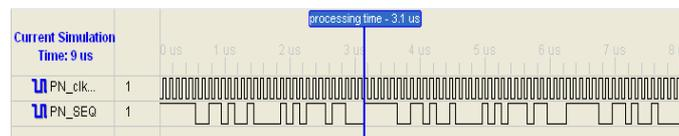
Figure 4: Simulation Results of PRBS generation
